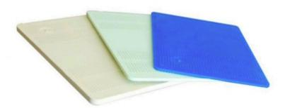
All CONAC Plastic Shims come with a non-skid surface with rib patterns, thereby increasing the coefficient of friction and preventing slippage while aligning panels. CONAC Plastic Shims are colour coded by the thickness and come in two different sizes: full size or half size. Therefore, size selection and identification becomes easy.
